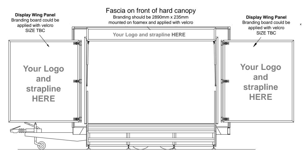
Overall length when full deployed 5520mm Overall width 3550mm including canopy
